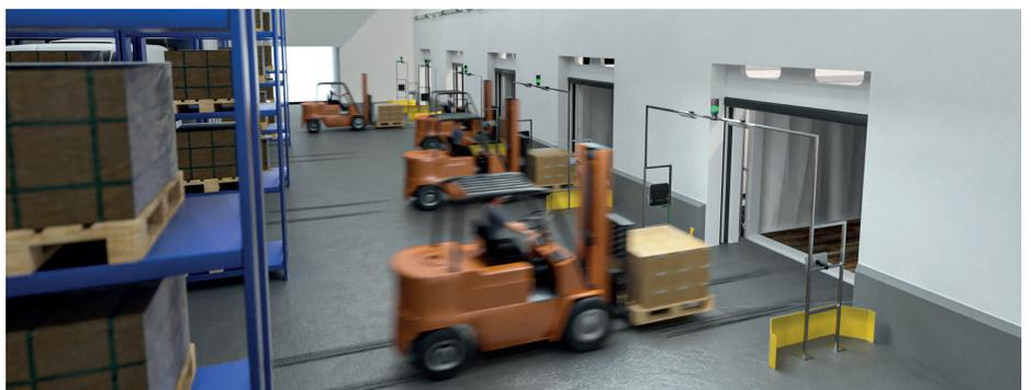
operation of the read/write head responds alternately to the antennas and thus ensures fast recognition of all tags on the pallets. They are reliably detected even when the forklift passes quickly and regardless of the position and distance of the tags to the read/write head.
