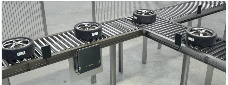
These can also be used for the exclusive acquisition of tags in the vicinity of the antenna. Since the read/write head recognizes which antenna has read a certain tag, the position of components on product carriers can also be easily determined.
